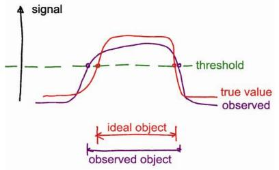
Fig. 7. Error in observation of property results in error of object boundary
