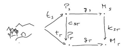
Photographs of smaller scale may be produced from larger scale photographs by the filtering operation  $c_{ST}$  thus  $M_T$  can be produced without taking the photograph at scale T
